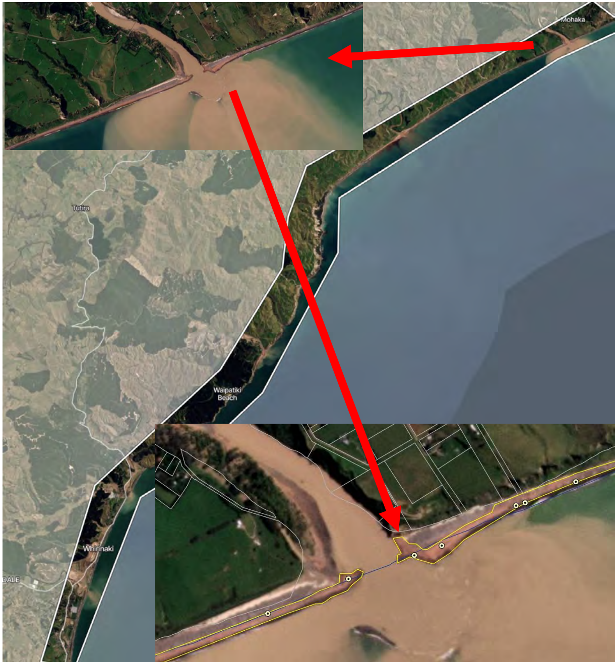
Figure 2 - Example of extracted coastline from imagery gathered on 20 February, with enlarged view of the Mohaka River mouth, and example of mapping the woody debris area (yellow polygons) impacted on the beach. Randomised sample locations are also shown (yellow circles).
