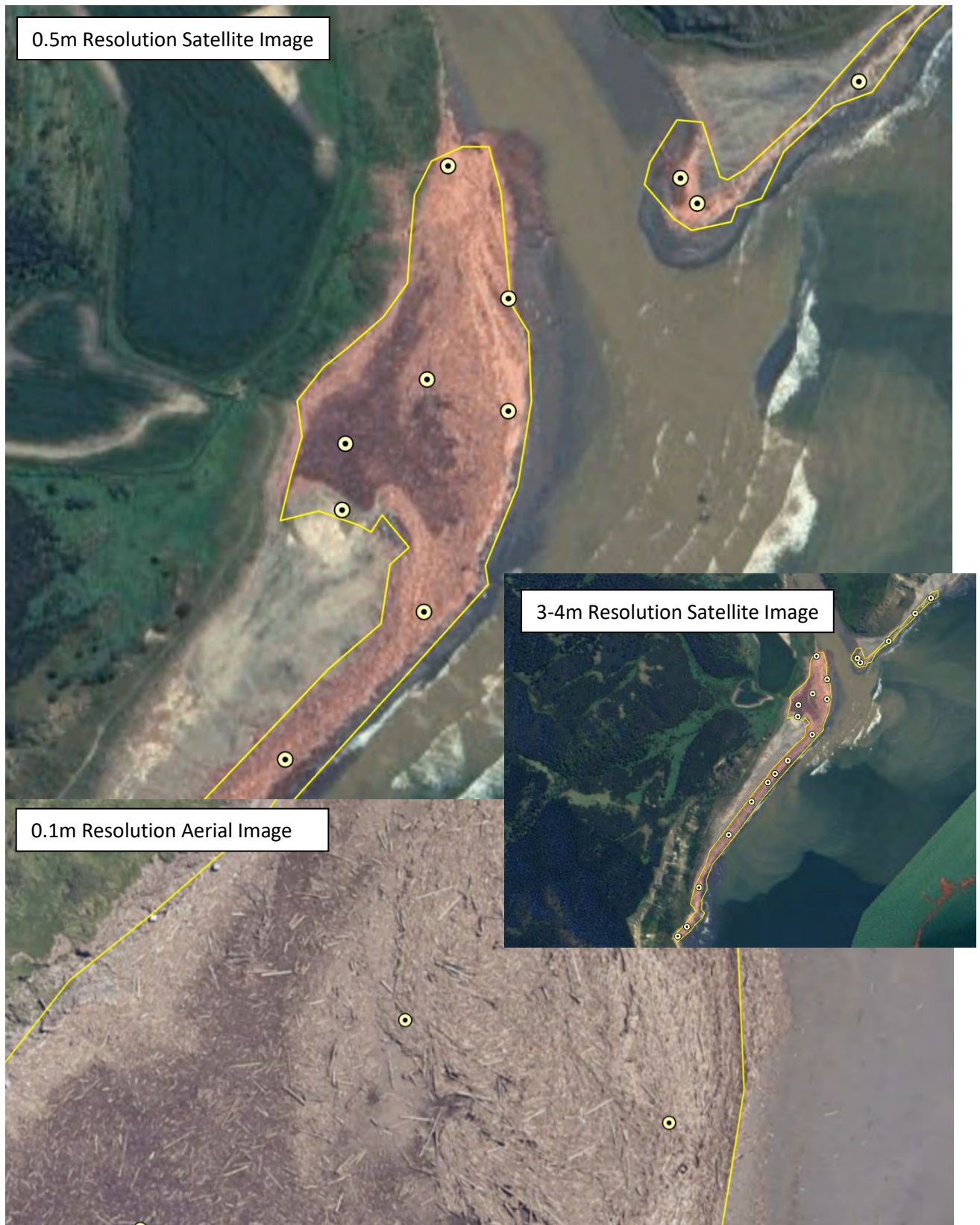
Figure 3 – Validation of woody debris mapping using varying resolutions of imagery, 3-4m GSD Planet, 0.5m (LINZ 2023A) provided satellite imagery, and 0.1m aerial imagery (LINZ 2023B) of the coastline of Aropoanui Beach showing woody debris accumulation (yellow), and sample plots (yellow points).
