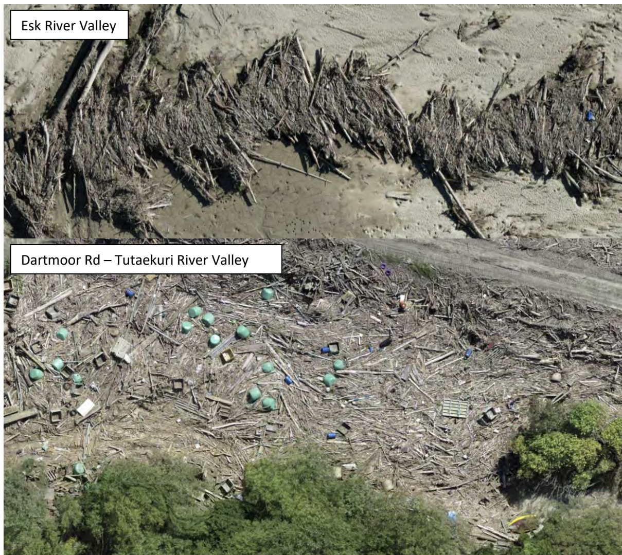
Figure 4 – Examples of drone imagery used to document discreet woody debris piles in various locations in river catchments around Hawke’s Bay.
