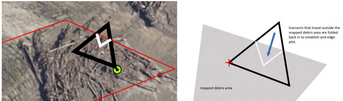
Figure 18 - Edge plot mirage methodology for narrow debris piles or where transects fall into areas outside of the mapped debris extent.
